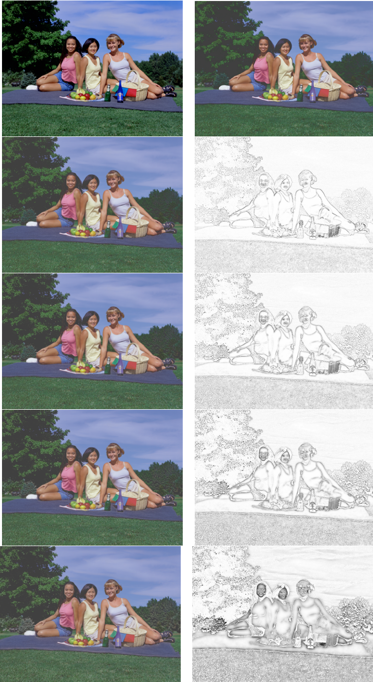
Fig. 3. Original (top left) and gamut clipped (top right) image, resulting image (left column) and \alpha_s (right column) for running the proposed algorithm with 2, 5, 10, and 50 iterations of the algorithm (top to bottom)
