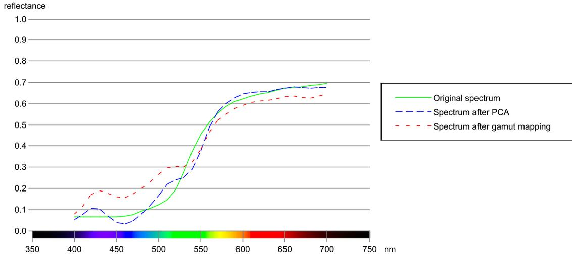
**Figure 4.** An illustration of a reflectance curve after gamut mapping has been applied in a 5-dimensional PCA space. The original spectrum is changed by the PCA transform as well as the gamut mapping.
