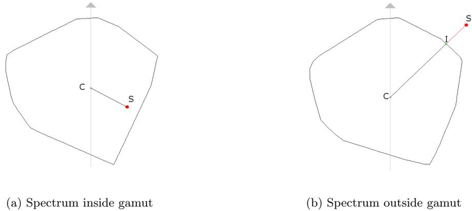
**Figure 1.** Cross sections of the spectral gamut. An outline of the device gamut is displayed, along with the gamut center (C) and the position of two spectra (S) which should be reproduced. The intersection (I) between the gamut boundary and the line from the center to the reflectance is found.
