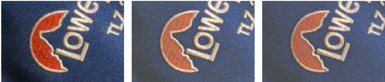
Fig. 15. Detail of the camera image; original, simple multilevel scheme (1) and the proposed algorithm of Table II.
