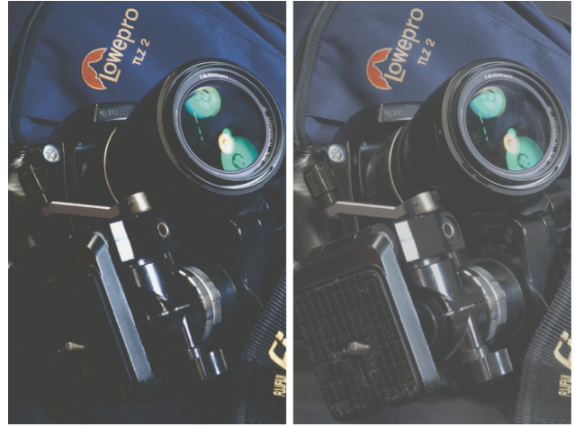
Figure 6. Gamut clipped image and spatial gamut mapped image using the STRESS algorithm.
