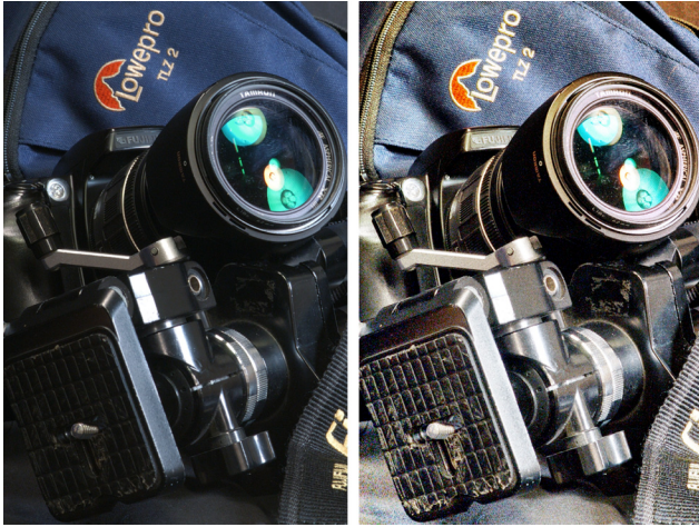
Figure 3. The STRESS algorithm applied to the color image on the left. The image size is 512 \times 779 pixels, and the parameters used were R = 300 , M = 3 , N = 100 .
